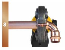
Line up the jaw of the tool so the centre of the jaw lines up with the raised section of the fitting.
