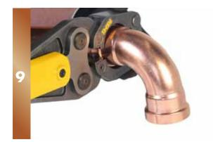
Place the adaptor jaw over the pins on the collar, check that the fitting is still matching up to the insertion depth mark on the tube. Press the trigger on the tool and hold down until piston retracts.
