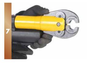
Insert the correct size press jaw for the size of fitting being pressed. Ensure jaw is clean and moves freely.
