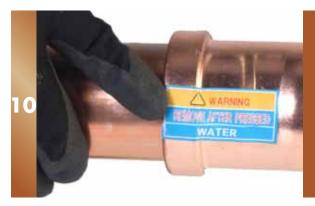
Remove the adaptor jaw from the collar, then the collar from the fitting. Now you can remove the sticker from the fitting to confirm press is complete.
