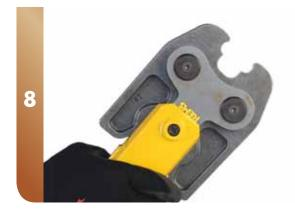
Place the adaptor jaw in the tool and ensure pin is pushed into place to hold jaw.
