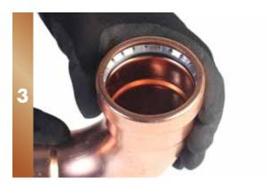
Check fitting to ensure it is suitable for the application. Confirm that fitting is clean and the O-ring and stainless grip ring are free from debris.
