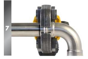
Line up the jaw of the tool so the centre of the jaw lines up with the raised section of the fitting.
