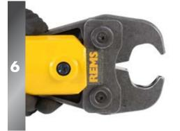
Insert the correct size press jaw for the size of fitting being pressed. Ensure jaw is clean vand moves freely.
