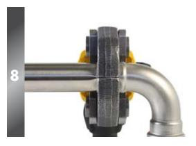
Press the trigger on the tool, hold down until jaws fully close and an audible click is heard. This completes the pressing process.
